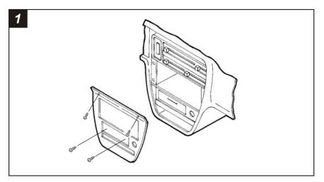
Disconnect the negative battery terminal to prevent an accidental short circuit. Remove the ashtray and (2) Phillips screws exposed. Remove (2) Phillips screws above the radio opening. Unclip the radio trim bezel and disconnect the cigarette lighter wiring. Remove (2) screws securing each side of the factory head unit and (1) screw from the rear support. Slide the unit out and disconnect the wiring.
